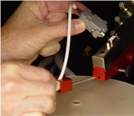
Use the L-4PQM to mount the SP4 and HT4 probe heads to any late model Lucas / Signatone Corp. resistivity test stand.
