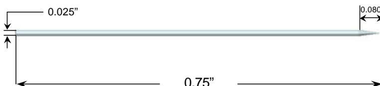
The SE-S may be used with the "S" & "P" Signatone probe tip holders. Typical Use: Probing hard surfaces or scratching through passivation.
