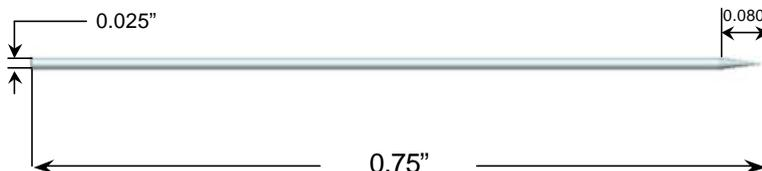
The SE-O may be used with the "S" & "P" Signatone probe tip holders. Typical Use: Probing Soft surfaces for good contact
