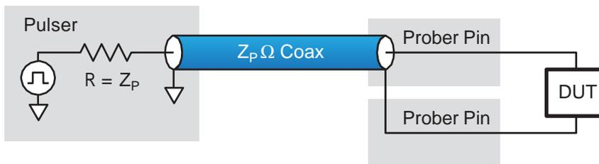
Figure 3: Pulse testing connection scheme for Kelvin connections.
