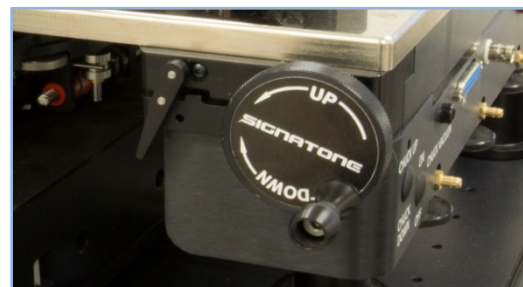
Platen “Fine Adjust” and “Position Lock”
