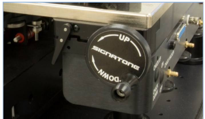
Platen “Fine Adjust” and “Position Lock”
