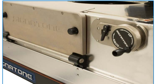
Platen “Fine Adjust” and “Position Lock”
